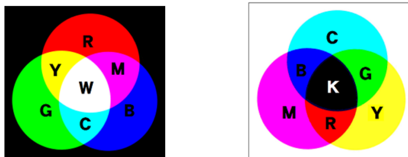
Figure 4. The three primary colors of light (left) and the three primary colors of color (right) (R: Red, G: Green, B: Blue, C: Cyan, M: Magenta, Y* Yellow, W: White, K: Black)
